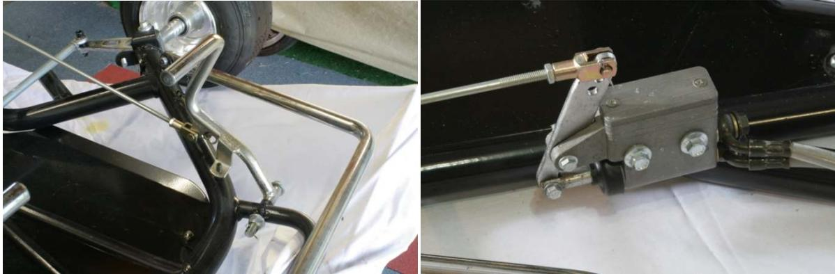
**Brake Rod** 3 Pieces (1x Brake Rod, 2x Brake rod brackets -May be supplied assembled)
