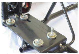
**Engine** 1 Piece Assembled \*BOLT KIT = Engine Fitting Kit (Contains: 4x Loop end M8 Bolts, 4x Nylon Spacer Washers, 4 Spacer Reinforcement Rings, 4x M8x50 Hex Head bolts, 8x M8 Nylocs, 8x M8 Washers, 4x Large Diameter M8 Washers, 1x M8 Throttle Cable mount, 1x Throttle cable terminating clamp).
