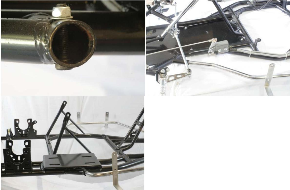
**Sidepod Bars** 2 Pieces \*FIT KIT = Contains 2x M6x40mm bolts, 2x M6 Nyloc Nuts & 2x 6mm Machine Washers
