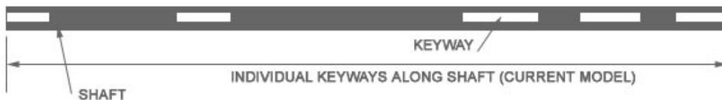
The axle shaft has keys set in different locations for 4 stroke or 2 stroke use. For four stroke use (in-board sprocket), you will not require the keyway second from the right. Orient your axle assembly so that when you look at the rear of the kart, it is set as per the diagram above.
