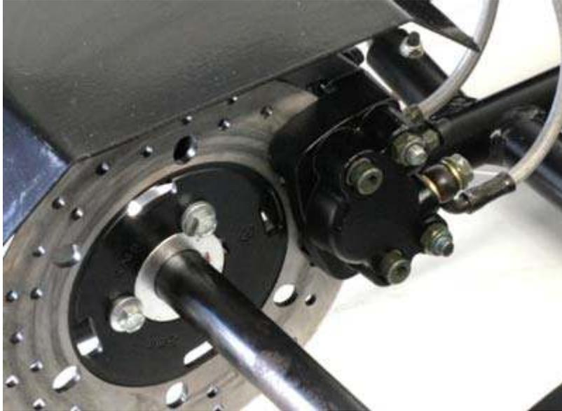
**Hydraulic Brakes** 1 Piece assembled (Master, 2x Lines, Calliper). \*RECOMMENDED FIT KIT Contains: 3x Zip Ties, 2x M8x50mm Square Head bolts, 2x M8 Nylocs, 2x M8x20mm Square Hex Socket Head bolts, 2x M8 8mm Spacers, 2x M8 Washers
